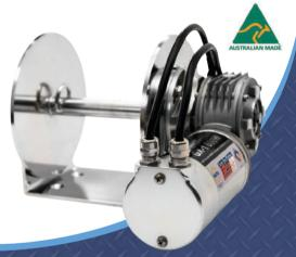
SPEC: 200MM DRUM 24MM SOLID SHAFT 88MM GEARSET 600W MOTOR MAX DROP-RETRIEVAL SPEED: 39M/126 FT. P/M HOLDING AT ANCHOR: 3T ROPE/CHAIN CAPACITY: 60M X 6MM ROPE + 5M TOPSHOT, 7M X 6MM SL CHAIN RECC. BOAT SIZE: 4-6M PACKAGED WEIGHT (APPROX.): 17KG
