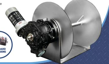
SPEC: 550MM DRUM 55MM SOLID SHAFT 220MM GEARSET 3250W MOTOR (24V ONLY) MAX DROP-RETRIEVAL SPEED: 50M/170FT P/M HOLDING AT ANCHOR: 11T ROPE/CHAIN CAPACITY: 150M X 20MM ROPE 13M X 13MM SL CHAIN RECC. BOAT SIZE: 15-20M+ PACKAGED WEIGHT (APPROX.): 130KG
